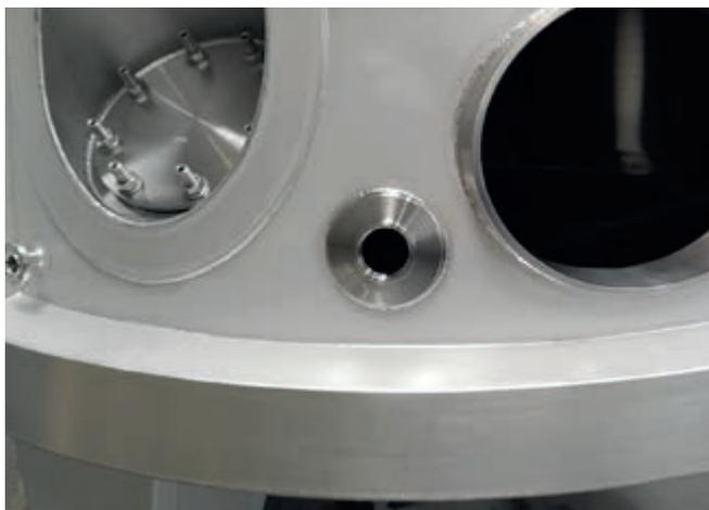
Tank welding flanges are welded into the tank wall or the tank bottom.
