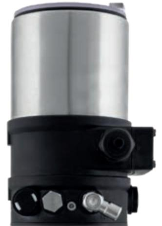
The digital positioners are part of the standard equipment of KIESELMANN control valves with reciprocating and membrane actuators. They are characterised by high control accuracy. The positioners operate in the signal range from 4 to 20 mA. However, they also control in the partial range or split-range operation.
