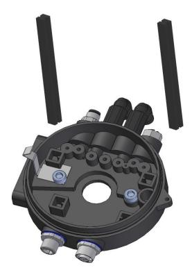
The magnets on position A are dislocated upwards by 3mm. This modification is very important in order to guarantee the recognition of the lower final position.
