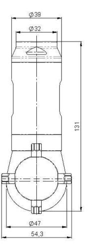
The dimensions can vary according to connection thread and nozzle diameter.
